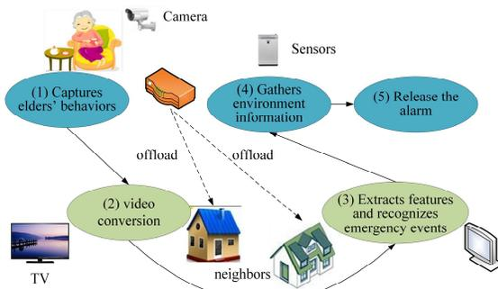
Fig. 2. An example service of home-to-home cloud. The domestic user offloads some tasks to consumer devices in neighboring houses.
