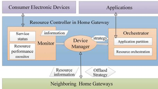
Fig. 4. Resource controller inside a home gateway. Three functions, device manager, monitor and orchestrator are contained.
