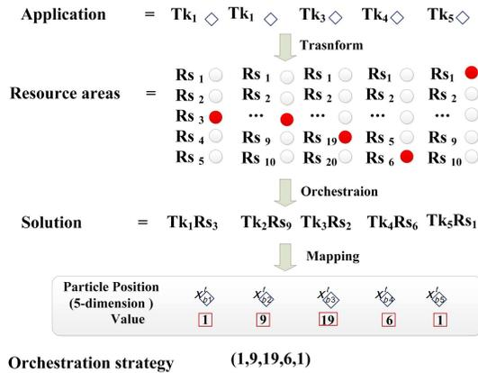
Fig. 7. Mapping resource orchestration to discrete PSO.
