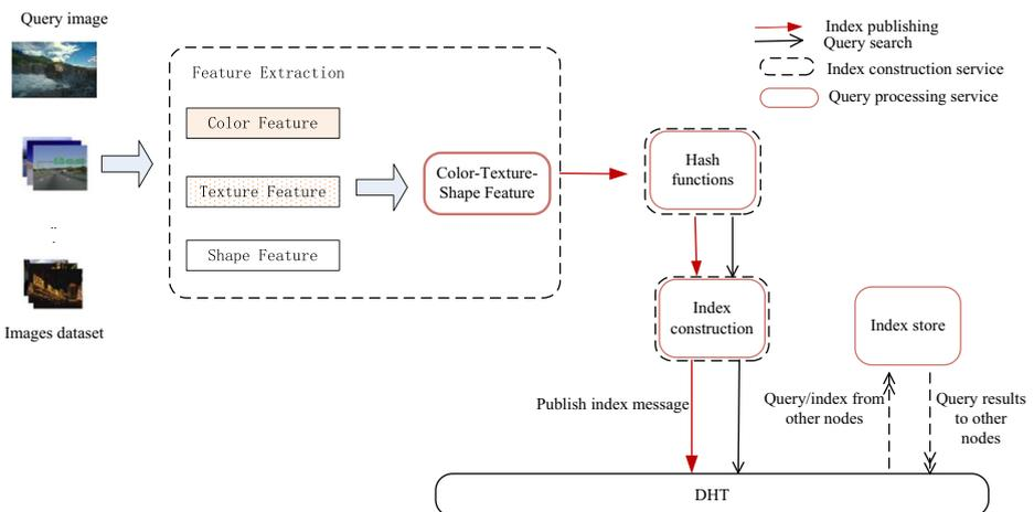
**Fig. 2** Components of a LFFIR node
