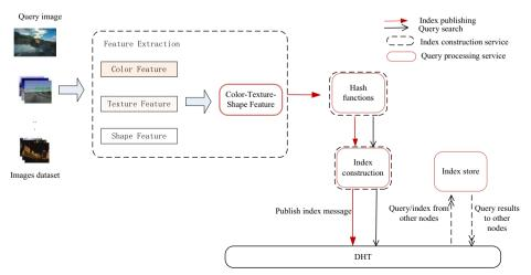
Fig. 2 Components of a LFFIR node
