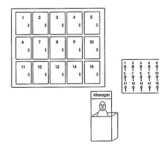
Each key has a number which corresponds to the number of the locker it opens. The dynamic memory area is very similar to a left-luggage room, where memory cells are lockers and memory addresses are locker keys; as each locker can be opened with its key, a cell can be accessed by its associated memory address. Notice that neither keys nor memory addresses can be modified (both are literal values).
