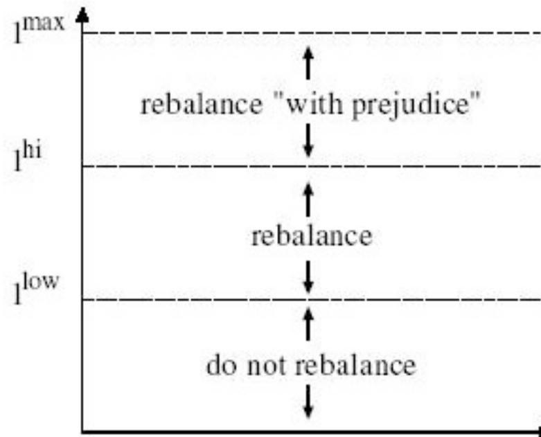
Figure 3. The server capacity is  $l^{max}$ . Load is sometimes re-balanced if greater than  $l^{low}$ , and always if greater than  $l^{hi}$ .
