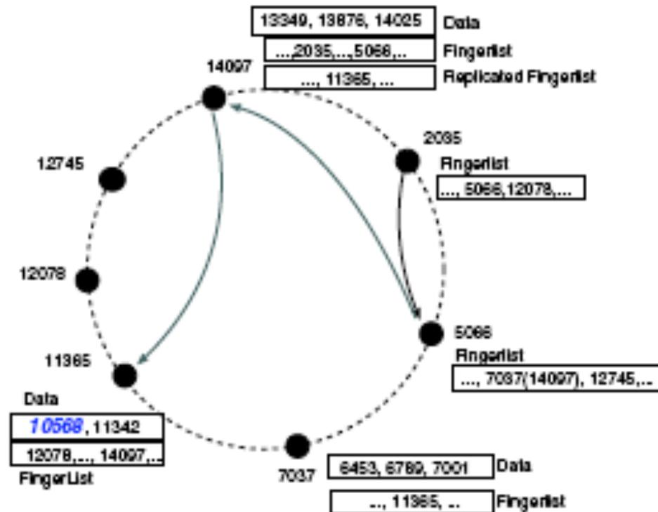
Figure 5. LAR routing and replication in Chord
